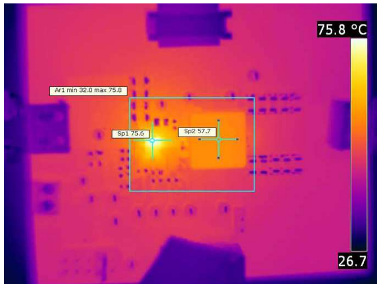
Figure 39. SP1: 75.6°C (TPS53915), SP2: 57.7°C (Inductor)
